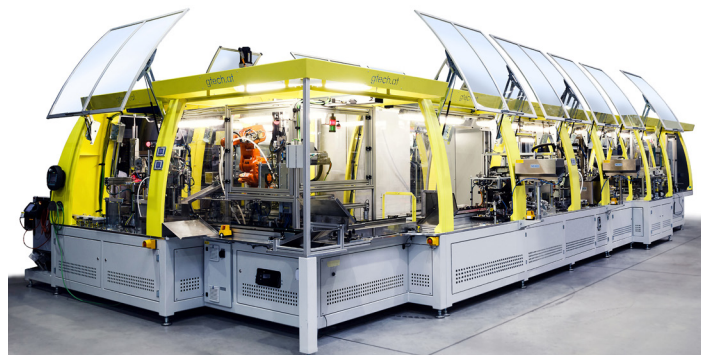
Fig: In this fully automated mounting facility, water pumps are mounted for a German automotive manufacturer in 18-second cycles.
